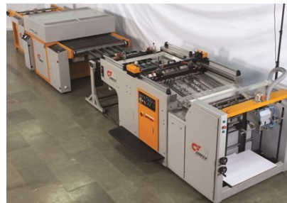
CYLINDER PRESS USES TUBES WHICH CONTINUOUSLY ROLLS AND PRINTS THE IMAGE THAT HAS BEEN WRAPPED AROUND IT.
