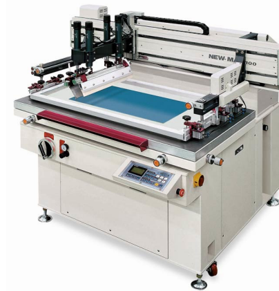
FLAT-BED PRESS USES A SQUEEGEE THAT PRESS AGAINST A MESH TO PRINT THE IMAGE.
